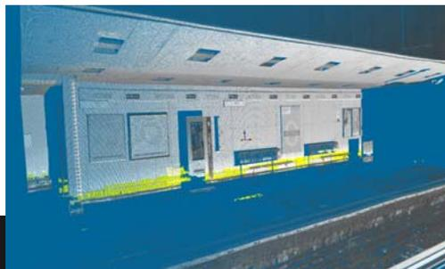
*Laserscanning can capture point data from the track very rapidly, as these scans demonstrate. The image on the right which has been rendered is of a station, whilst that below shows the track and a train. The hard work comes in thinning the data to get usable profiles.*
