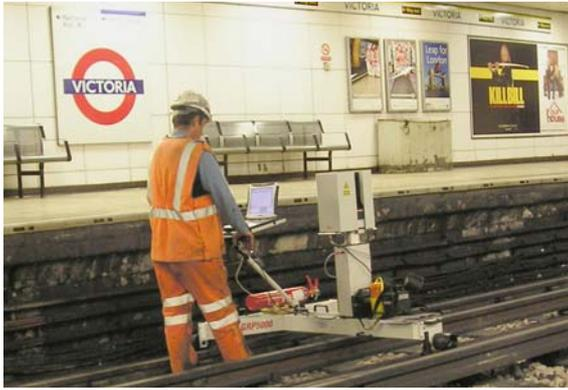
**ABA Surveying are using Laser-scanning to capture gauging data ahead of new rolling stock on the London Underground.**
