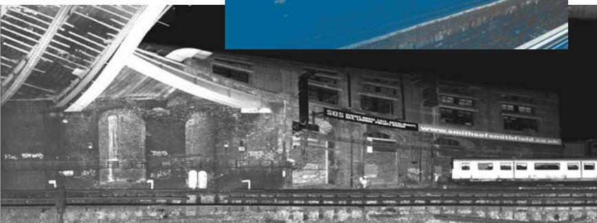
The aspects of data that the geospatial surveyor is required to collect primarily relate to the track position, cant, radius and minimum clearance dimensions to trackside infrastructure that might impact on gauging. These are evaluated against rolling stock design parameters such as length of coach, the design envelope, the position of the wheels and the wheelbase, suspension characteristics and the design speed using a software package called ClearRoute.
