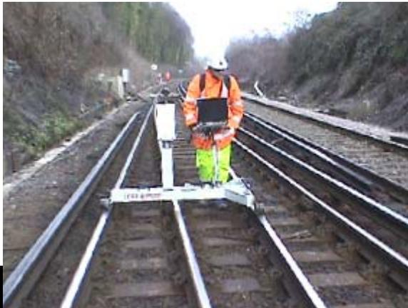
*On the open track the scanner measures and records all visible detail including trackside and overhead infrastructure. If it's in the scan it has been measured to millimetres.*
