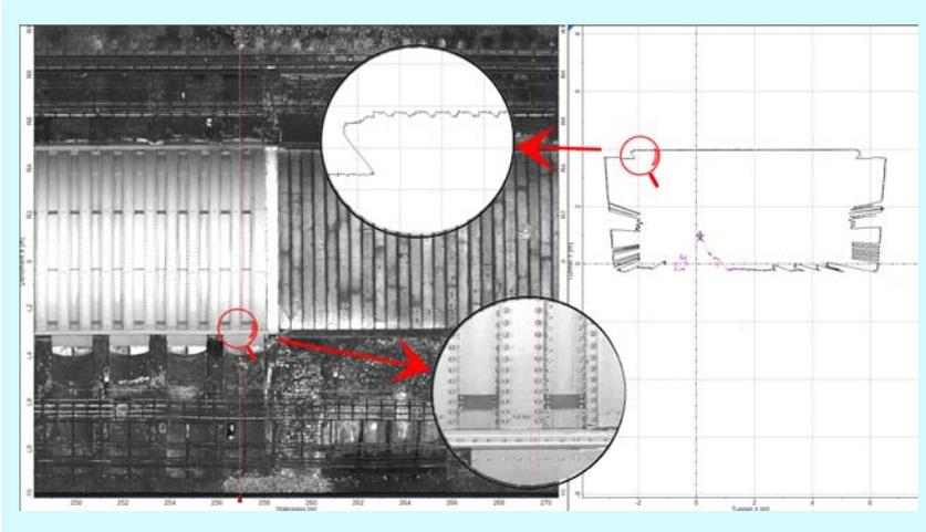
*No detail is too small that it does not get scanned. The image above shows how much detail from within a tunnel is captured.*
